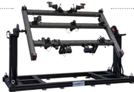
System for optical measurements
