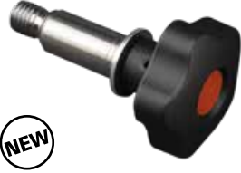
Fastening bolt, star knob, side mount, red, M10 / sleeve D11.98H7
